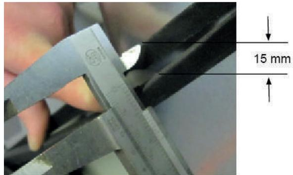
Tension of V-belt is ok, if a maximum measure of 15 mm can be held under light pressure on the front stretch on the V-belt.
