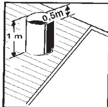
The opening of the flue pipe must not be near a window or a balcony.
