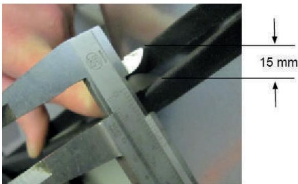
Tension of V-belt is ok, if a maximum measure of 15 mm can be hold under light pressure on the front stretch on the V-belt.
